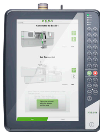
T150 SWL with robotics keyboard
